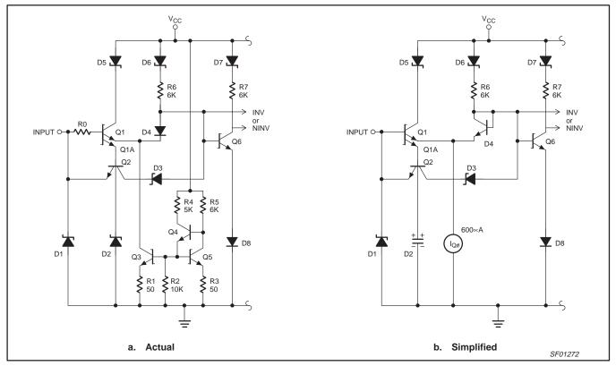
Figure 1. The "Light Load" and Speed-Up Circuit Input Structure (Actual & Simplified)
