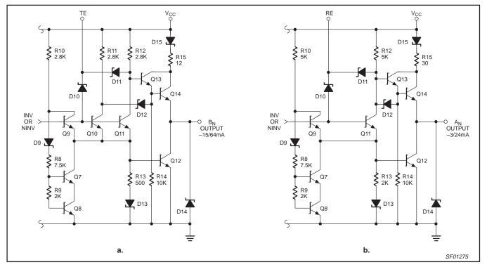
Figure 4. Two Typical "Light Load" Output Structures (74F657)
